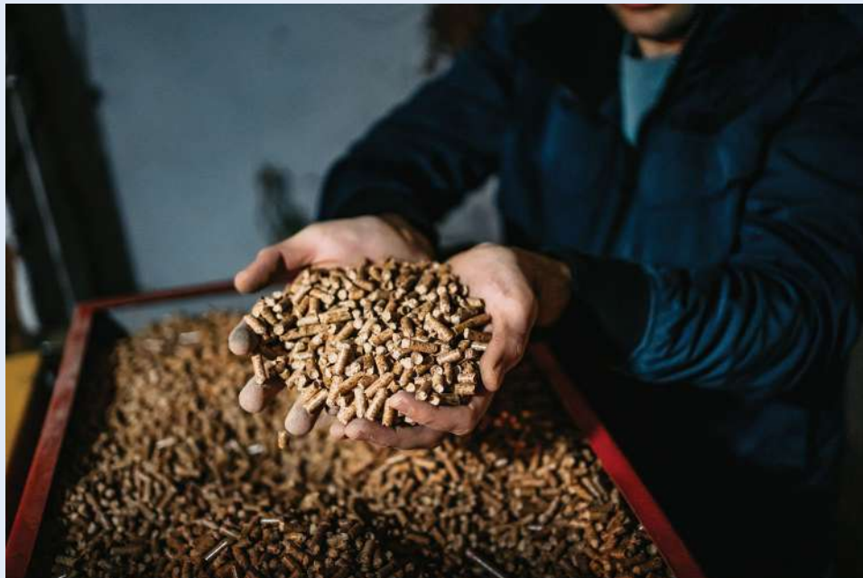
Figure 3.8: These biofuel pellets are made out of sawdust that has been compressed.
