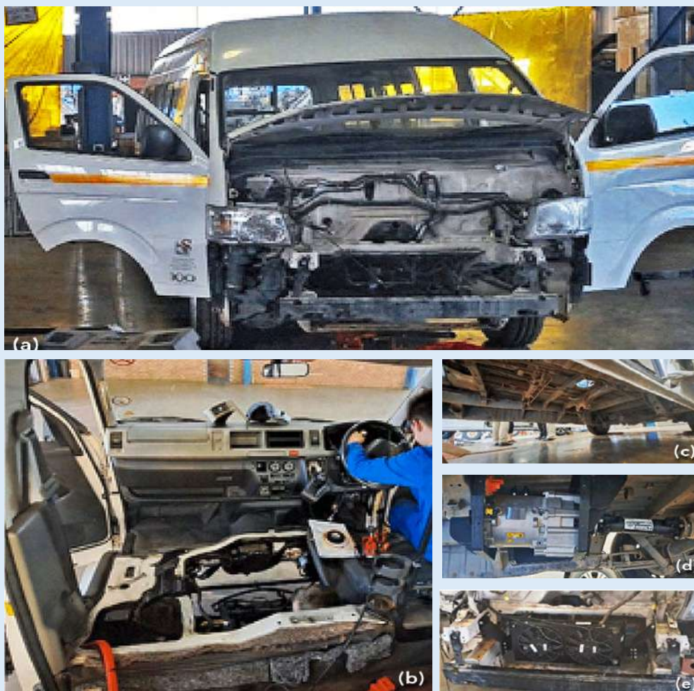
FIGURE 20. Vehicle with combustion-related components removed (a) Front view of the stripped vehicle. (b) Empty engine compartment. (c) Bottom view of stripped vehicle before electric motor and prop-shaft installation. (d) Electric motor with prop shaft (protective cover not shown). (e) Radiator for the electric motor coolant (Lacock, et al., 2023)
