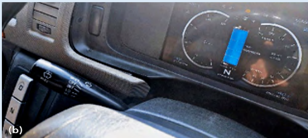
FIGURE 19. The electric retrofitted minibus taxi (original model from 2009) (a) Completed retrofitted taxi. (b) Retrofitted electric vehicle's electronic dashboard and controls (Drive (D), Neutral (N), Reverse (R)) (Lacock, et al. , 2023)
